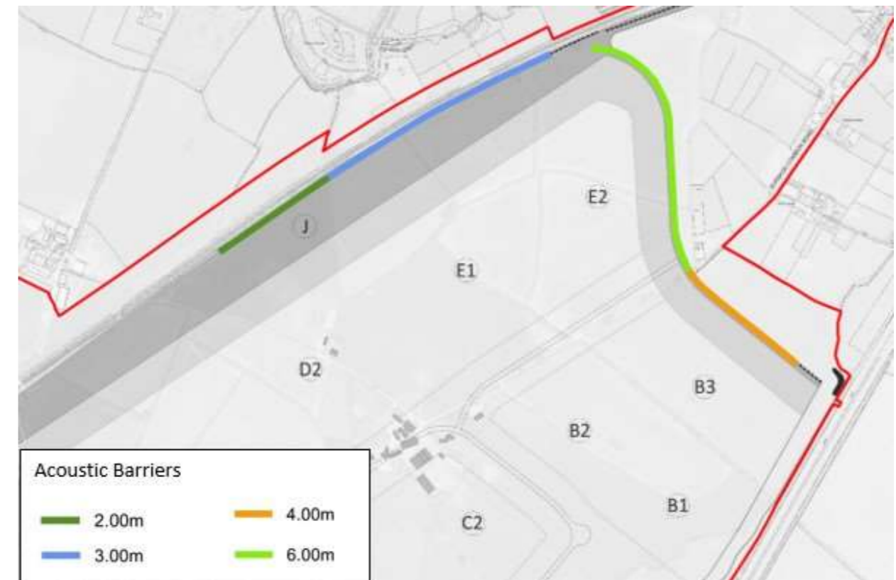
Fig. 61 Proposed Noise Barriers to north west of Railport and to the north east of head shunt (Document Reference 6.3.10.10)
